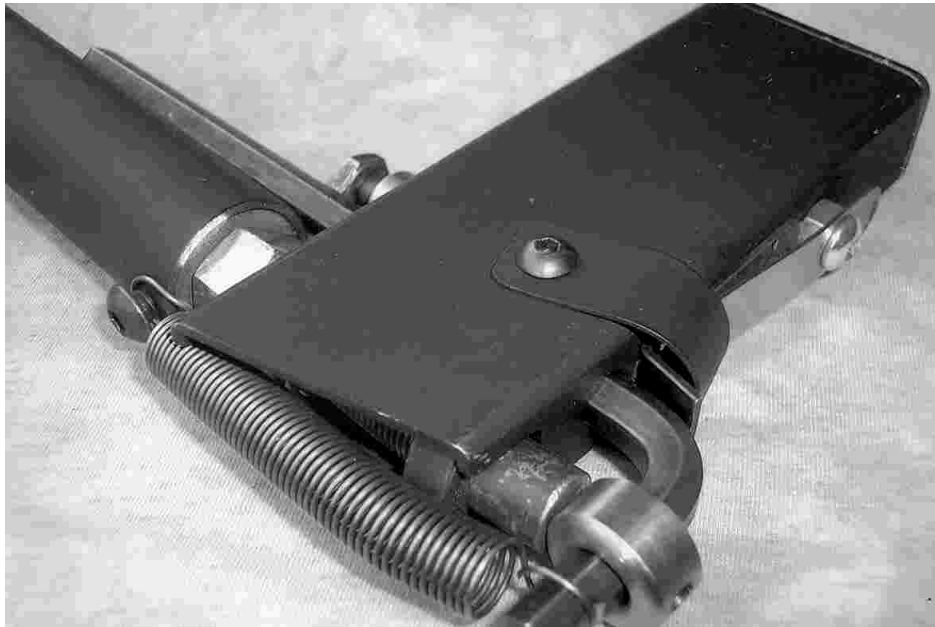
Close up of the striker and breech block.
